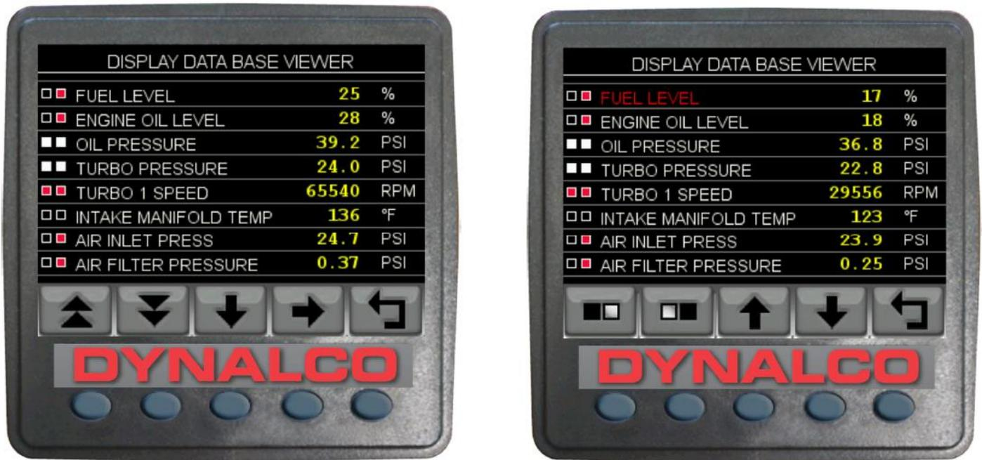
**LEFT:** This screen can be adapted to allow the data mapping / filter for each of the three data views. The operator can check boxes for each item they want to appear on each of the standard views (Quad and Single). Key 1 and Key 2 are page up/down respectively. Key 3 moves down the list one item and Key 4 is to edit the settings of the view filters. The red box indicates that the option is not available.
