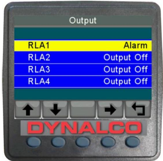
**LEFT:** This screen is used to turn ON and OFF relay alarms, if wired into the associated pins of the D-100 unit. These are open connector outputs, suitable for 0.5A continuous loads.
