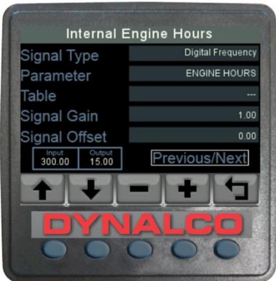
This screen is used to set up the internal engine hour meter.
