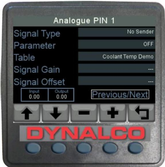
This screen is designed for configuration of analog pins. Use Key 1 and Key 2 to navigate up/down. Use Key 3 and Key 4 for back/forward.
