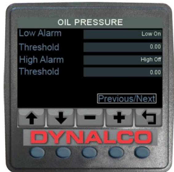
**LEFT:** This screen is used to access all alarms. That can be set for the analog pins, digital pins, internal voltage and internal engine hours.
