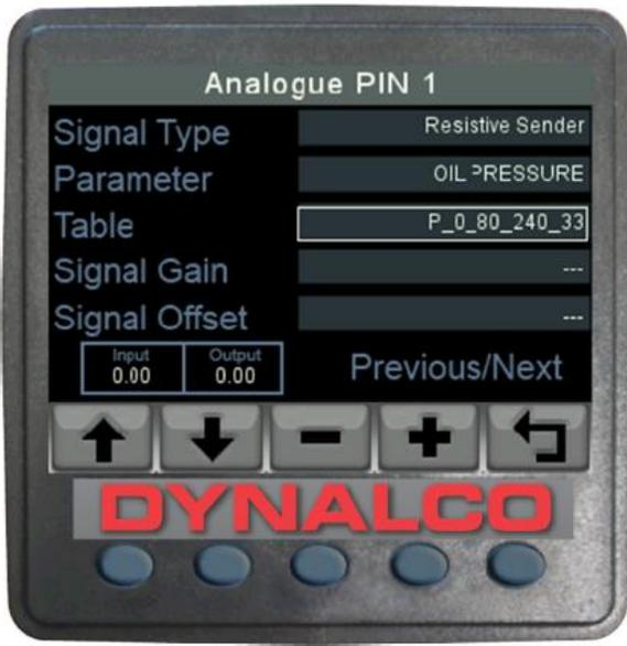
Example: This is an example of a 0-80 PSI oil pressure sender using the 240-33 ohm resistance range. The prefix:
