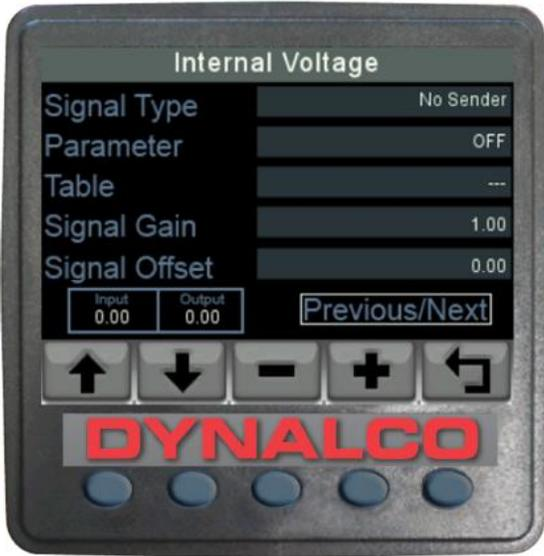
There is no pin for voltage; the voltage reading is extracted from the supply voltage of the D-100 unit.
