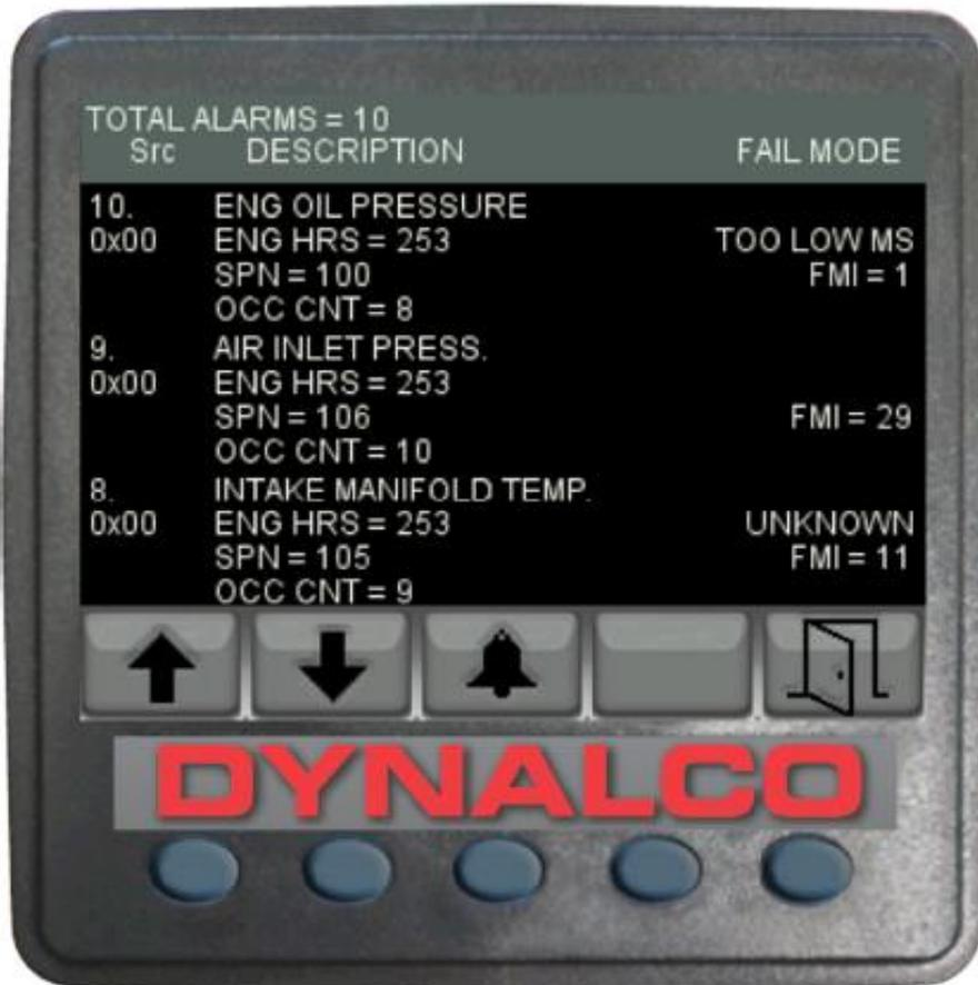
Typical Alarm Screen after Alarm Acknowledge
