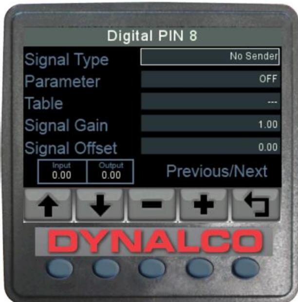
This screen is designed for configuration of digital input signals.
