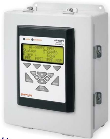
***The AF-900PC Air/Fuel Ratio Control System utilizes heated O<sub>2</sub> sensors and full-authority fuel valve control to precisely maintain the air/fuel ratio of rich-burn carbureted gaseous fueled engines.***
